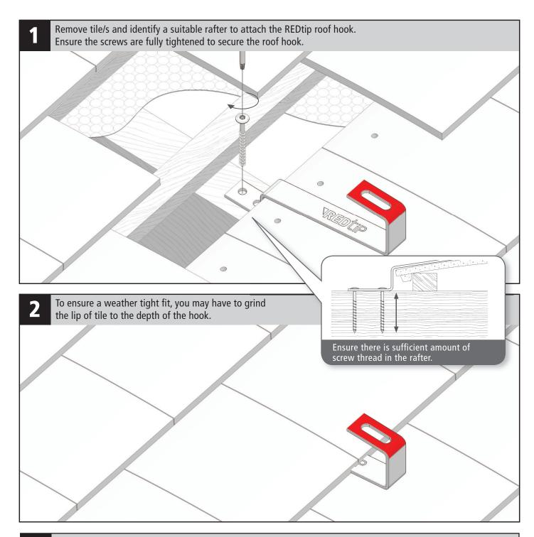
The distances between the roof hooks will be dependent on structural and wind loadings. Always consult a Structural Engineer if you are in any doubt.
